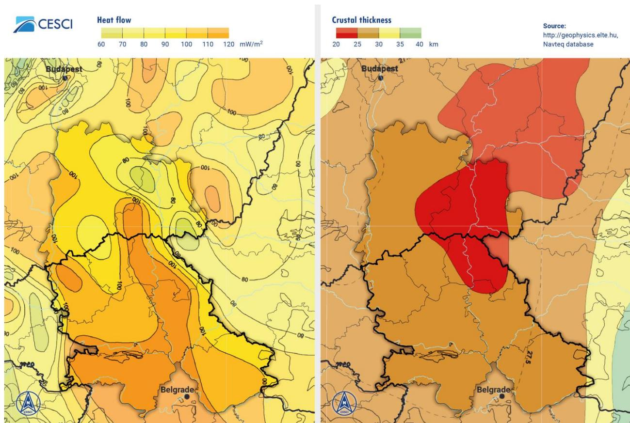
Geothermal energy is only partially renewable, but the Carpathian Basin's huge supply will most probably last for thousands of years. There is a geothermal system where the heat source, the reservoir and the transport fluid coexist. The reservoir is a hot, permeable rock volume, which the fluid circulating in it gets the thermal energy from, and which is constantly heated by the ground thermal flow. Geothermal fluid is mostly thermal water, which can be in the form of liquid or vapor,
