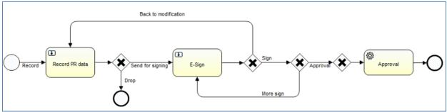
Fig.5. Recording workflow
